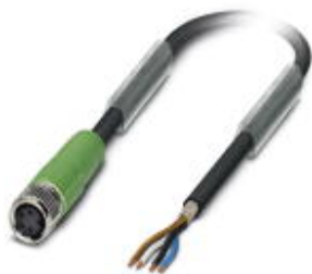
Sensor/actuator cable, 4-position, PUR halogen-free, black-gray RAL 7021, shielded, free cable end, on Socket straight M8, cable length: 1.5 m
