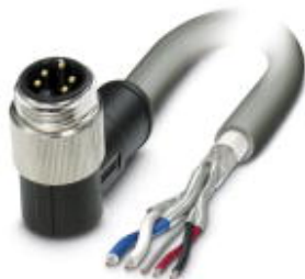
Bus system cable, DeviceNet, 5-position, PVC, Gray RAL 7001, Plug angled 7/8"-16UNF, on Free cable end, Cable length: 20 m
