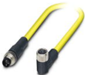
Sensor/Actuator cable, 3-position, PVC, yellow, Plug straight M8, on Socket angled M8, Cable length: 1.5 m
