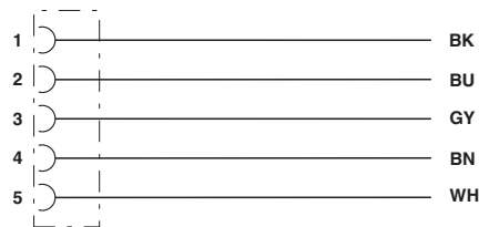
Contact assignment of 7/8" socket
