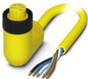
Power cable, 5-position, PVC, yellow, Plug angled 7/8"-16UNF, on free cable end, cable length: 10 m
