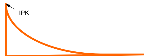
Figure 26. Input Charge Inrush Current
