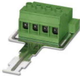
Plug component, Nominal current: 125 A, Rated voltage (III/2): 1000 V, Number of positions: 4, Pitch: 15 mm, Connection method: Screw connection, Color: green, Contact surface: Silver
