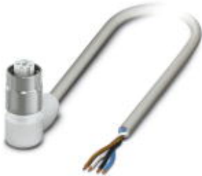
Sensor/Actuator cable, 4-position, PP-EPDM halogen-free, Gray RAL 7035, Free cable end, on Socket angled M12, A-coded, Cable length: 3 m, Hygienic design, With high-grade steel knurl
