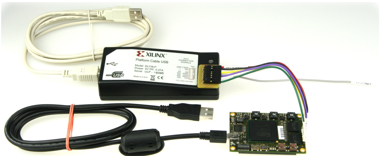
Figure 27: recommended TE0320 set-up.
