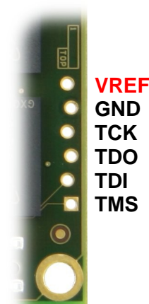
Figure 24: JTAG connector J2.
