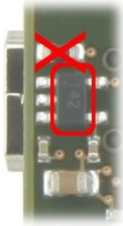
Figure 8: assembly option for VCCAUX = 2.5 V (bottom view).
