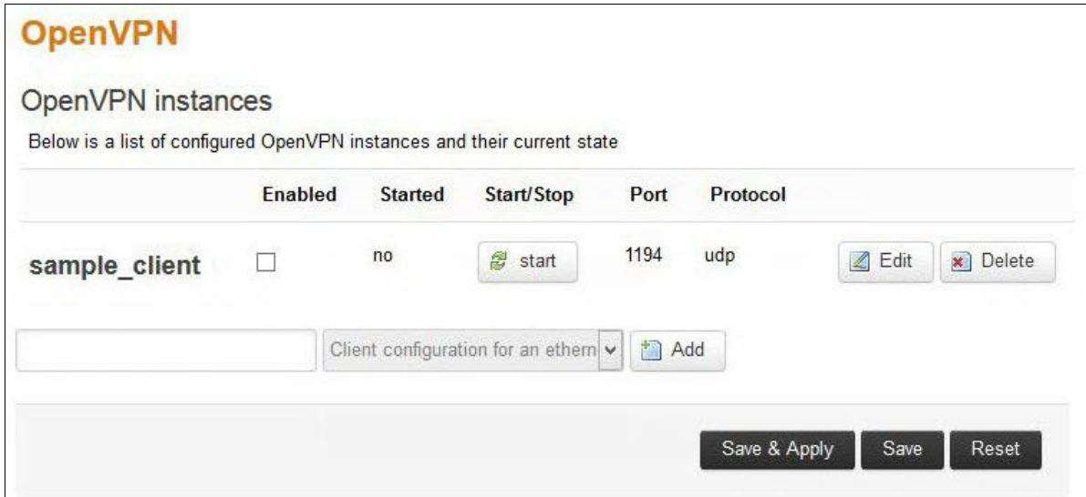
Screen 12-3: OpenVPN Service Configuration
