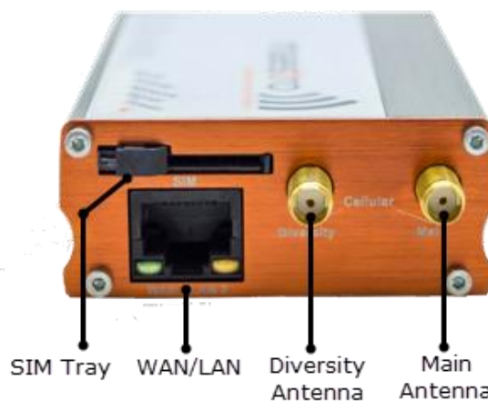
Figure 5.2-2: Maestro Router WAN Panel
