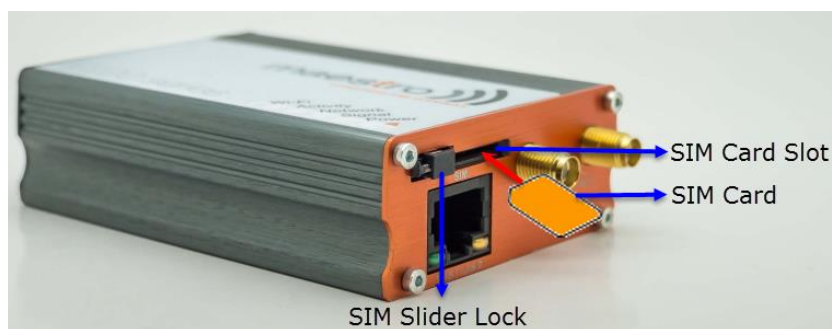
Figure 5.4-5: Insert SIM Card
