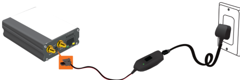
Figure 5.4-8: Connecting to AC receptacle
