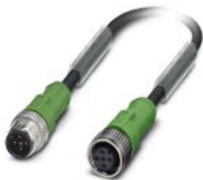
Sensor/actuator cable, 5-position, PUR halogen-free, black-gray RAL 7021, Plug straight M12, A-coded, on Socket straight M12, A-coded, cable length: 5 m
