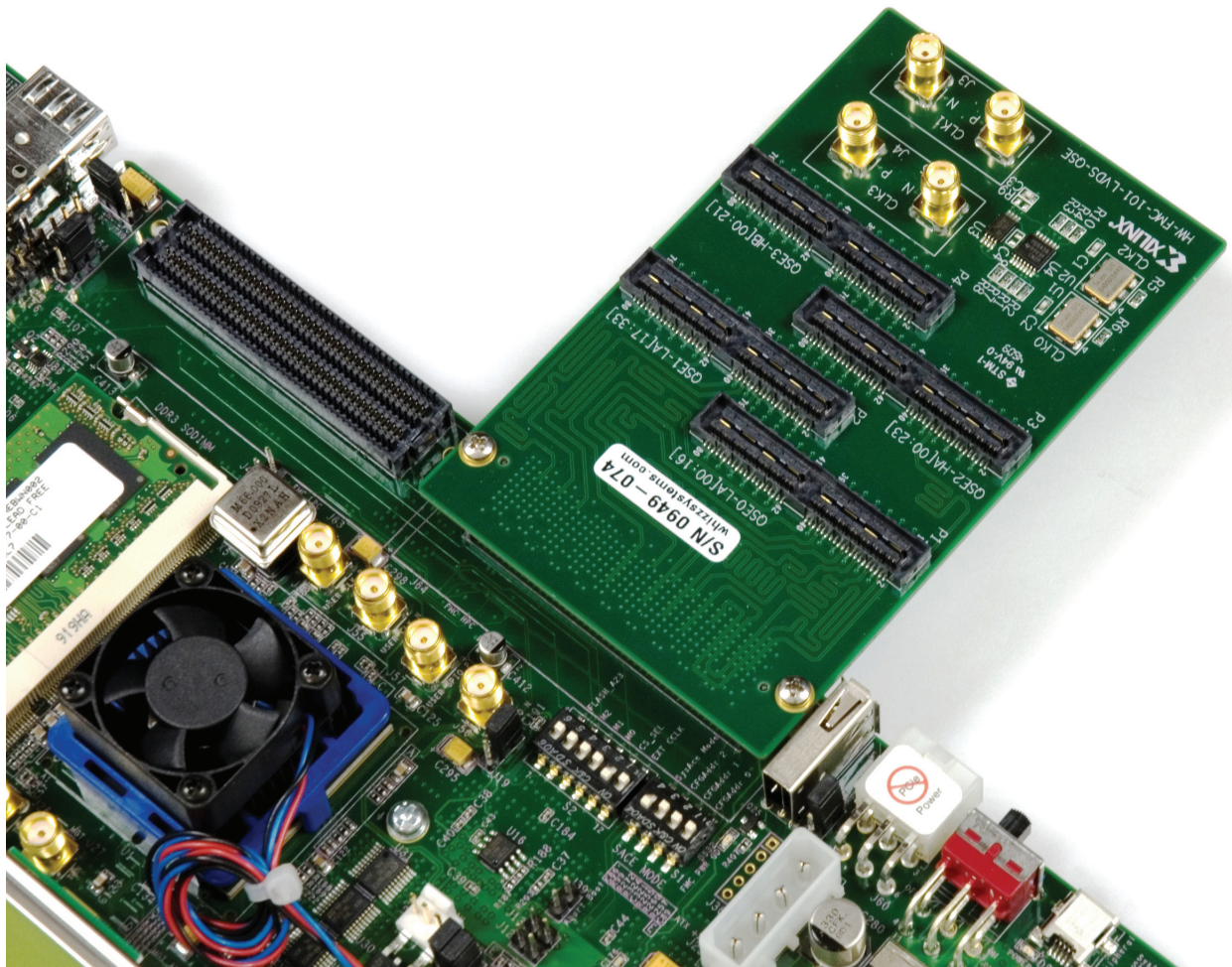
Figure 1-1: Installation of XM101 to ML605 Board FMC HPC Connector
