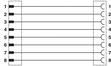
Contact assignment of the M12 plug and the M12 socket
