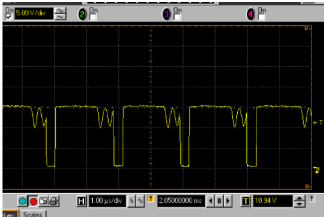
FIGURE 7. BOOST SWITCH NODE AT 100mA (PARTIAL DISCONTINUOUS)
