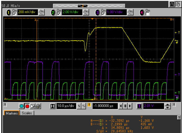
FIGURE 21. ENT BIT GOING HIGH TO TONE ENABLED ON THE OUTPUT DELAY IS \sim 34\mu\text{s}
