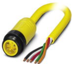
Power cable, 5-position, PVC, yellow, Plug straight 7/8"-16UNF, on free cable end, cable length: 1 m
