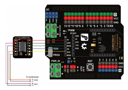
IO Expansion Shield V7.1 Connection Diagram
