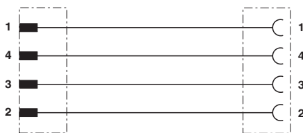
Contact assignment of M8 plugs / M12 sockets
