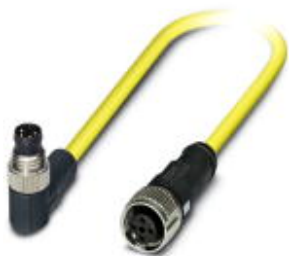
Sensor/Actuator cable, 4-position, PVC, yellow, Plug angled M8, on Socket straight M12 SPEEDCON, A-coded, Cable length: 0.5 m
