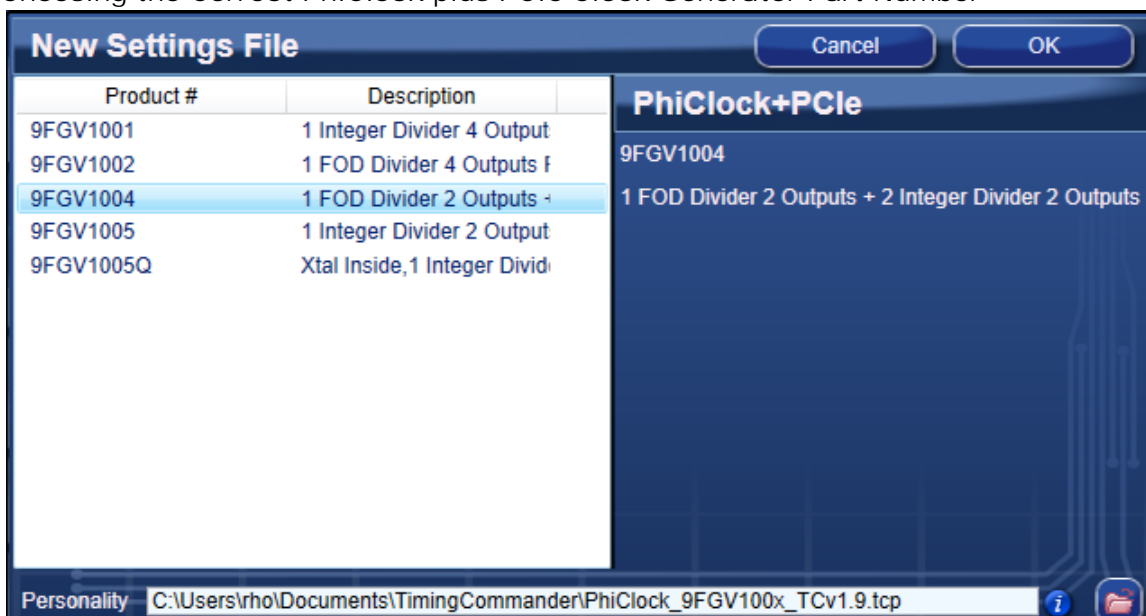
Figure 2. Choosing the Correct PhiClock plus PCIe Clock Generator Part Number
