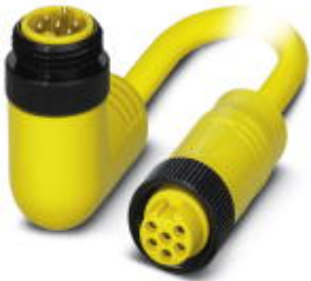
Power cable, 6-position, PVC, yellow, Plug angled 7/8"-16UNF, on Socket straight 7/8"-16UNF, cable length: 10 m
