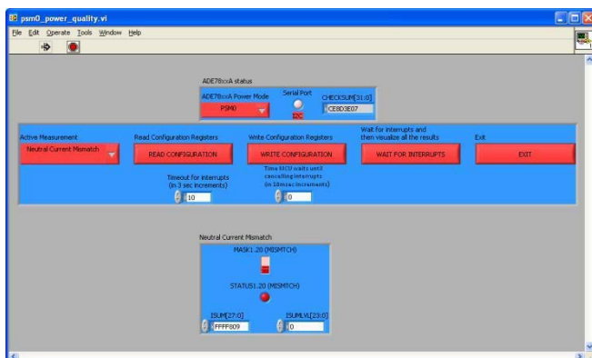
Figure 23. Neutral Current Mismatch Panel
