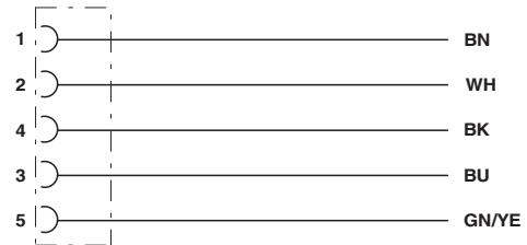
Contact assignment of the M12 sockets
