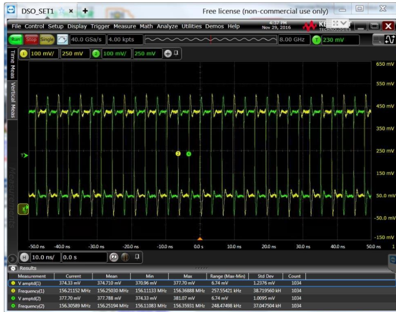
Figure 5-4. HCSL 1.8 V, 156.25 MHz Clock Measured with DC Coupling, 50-Ω Scope Termination
