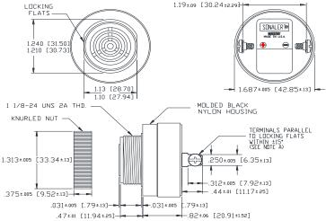
NOTE A: TERMINALS-.032 BRASS TIN PLATED, TAPPED FOR #6-32 SCREW. TWO #6-32 NICKEL PLATED BRASS SCREWS INCLUDED. WILL ACCEPT 1/4" QUICK CONNECT. NOTE B: MOUNTING- REMOVE BLACK PLASTIC NUT
