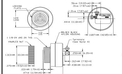
NOTE A: TERMINALS-032 BRASS TIN PLATED, TAPPED FOR #6-32 SCREW. TVD #6-32 NICKEL PLATED BRASS SCREWS INCLUDED. WILL ACCEPT 1/4\* QUICK CONNECT.
