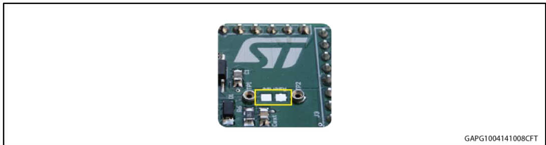
Figure 5: Pads for soldering SMD resistor
