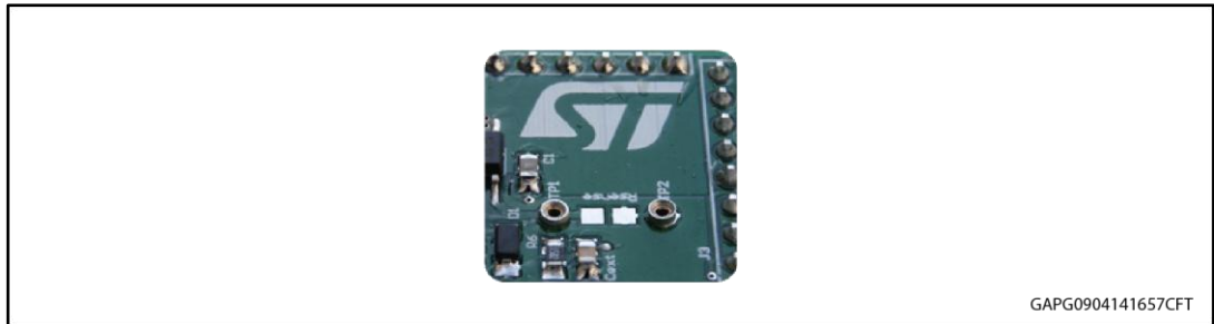
Figure 4: Mounting through-hole sense resistor
