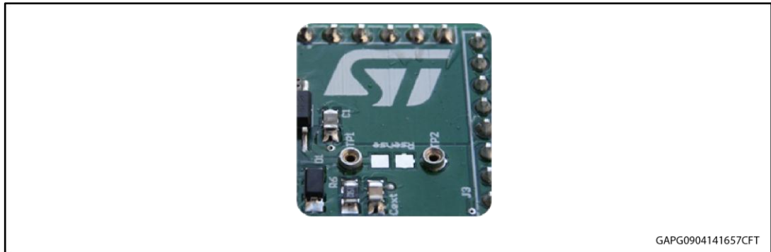
Figure 4: Mounting through-hole sense resistor
